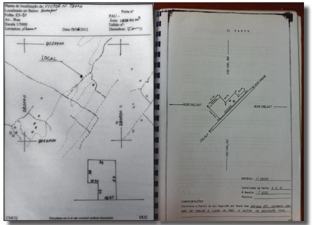
Figure 4 - Samples of two topographic surveys of two plots of land in Quelimane.
